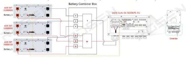
(4) Four pcs lithium battery connect diagram
