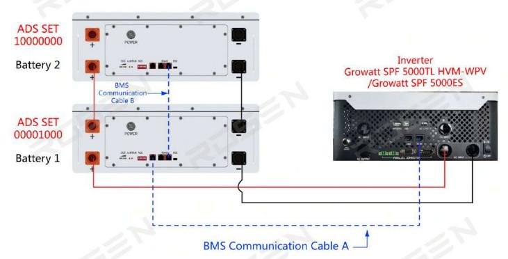
(3) Three pcs lithium batteries parallel connect diagram (E.G. Inverter : Growatt SPF 5000TL HVM-WPV/Growatt SPF 5000ES)
